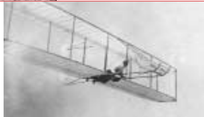
The 1902 glider, designed with the Wright's own wind tunnel data, was the first successful flying machine.
